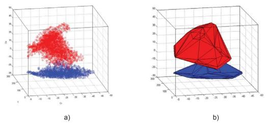
Figure 4: Selective distribution of the YCrCb color space: a – point presentation for scene, b – model of the convex hull
