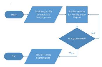
Figure 2: Block diagram of the software for image segmentation system
