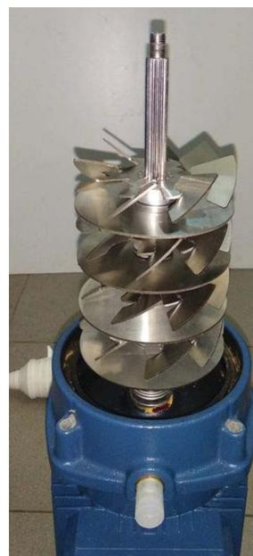
Figure 7: Photograph of the experimental rotor model
