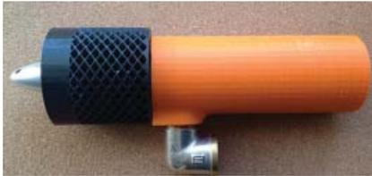
*Figure 8: Photograph of the experimental compressor (the orange compressor housing on the right) equipped with the experimental turbine (the turbine black mesh rotor on the left)*
