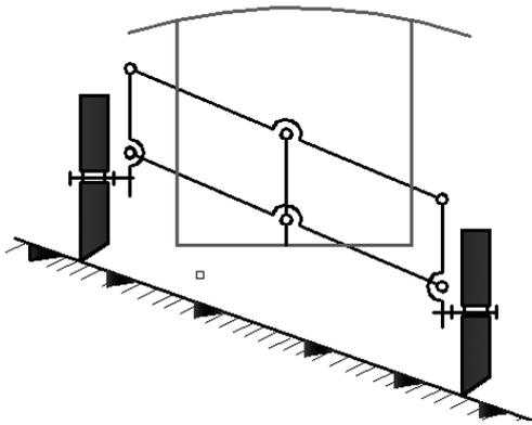
Figure 13: Scheme of vehicle undercarriage on horizontal supporting surface
