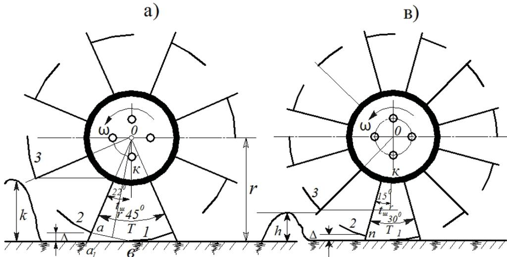
Figure 2: Diagram of eight and twelve-legged walking wheels
