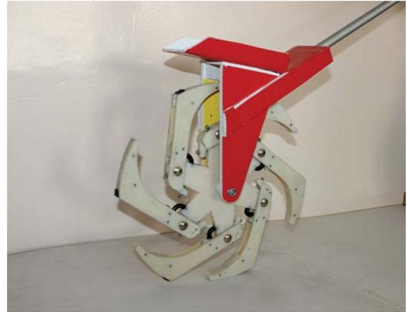
Figure 11: Picture of universal walking wheel model universal walking wheel, which was made to test certain properties of new wheel.
