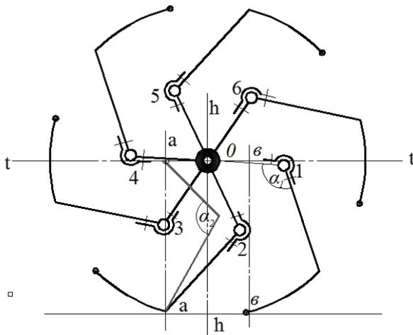
Figure 10: Diagram of universal walking wheel
