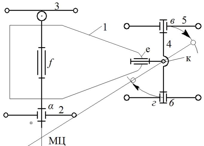
Figure 5: Undercarriage structural scheme when rotated
