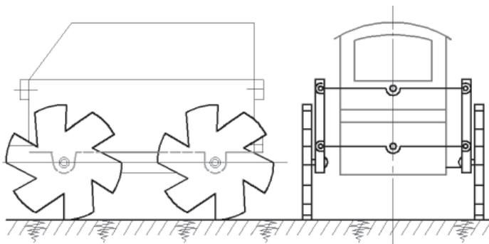
Figure 14: Scheme of vehicle undercarriage on inclined supporting surface
