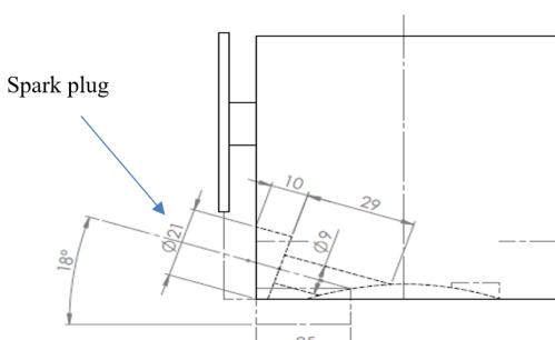
Figure 2: The placement of a modified spark plug angle
