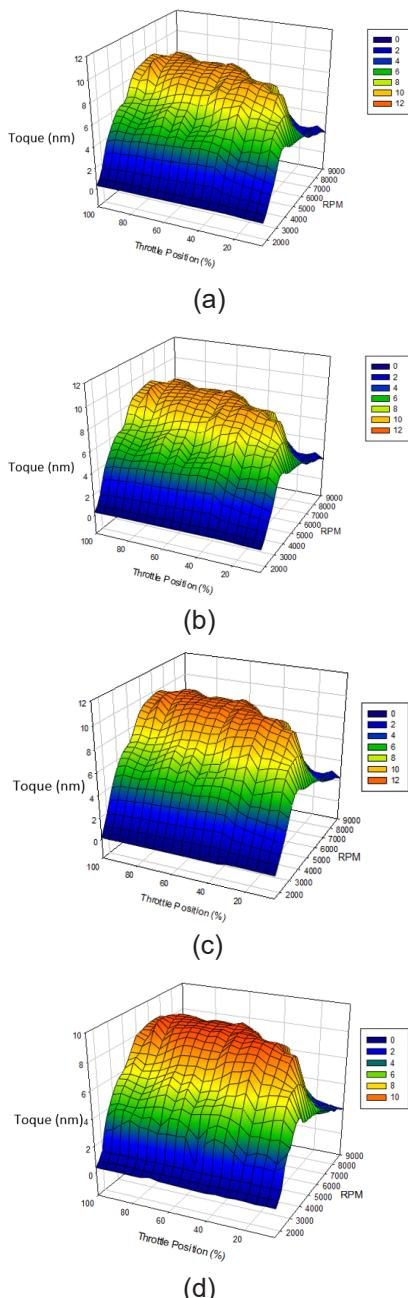
Figure 16: Resulted engine map for generated torque;
