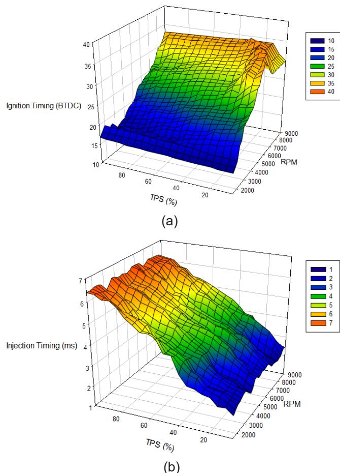
Figure 11: Ignition and injection timing; (a) Ignition timing map; (b) Injection timing map
