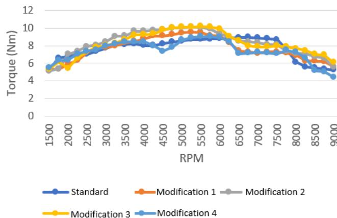
*Figure 14: Generated torque obtained from the engine test*
