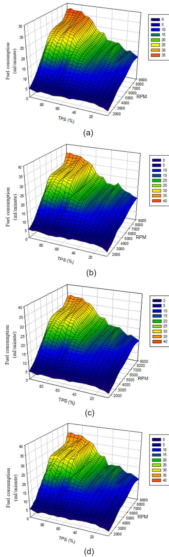
Figure 19: Fuel consumption rate: (a) Modification 1; (b) Modification 2; (c) Modification 3; (d) Modification 4
