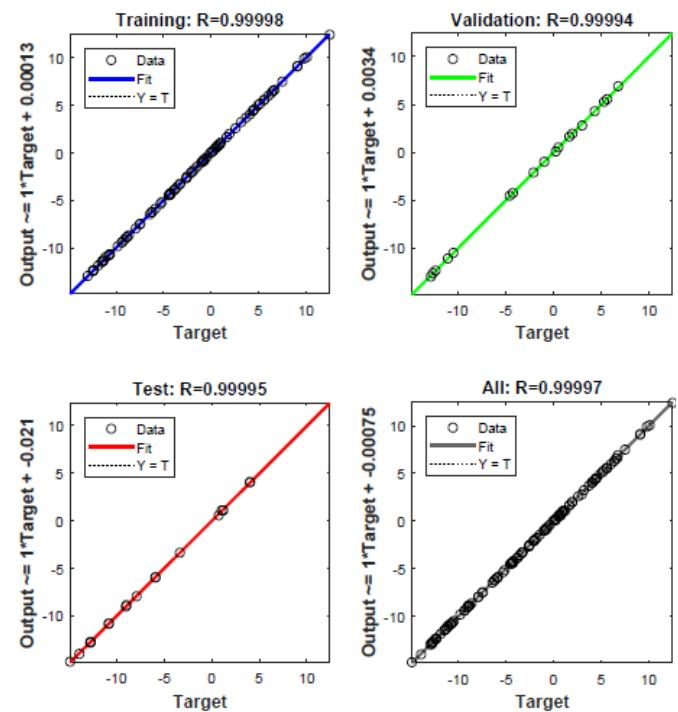
Figure 7: Selected neural network regression result of engine map for standard ECU
