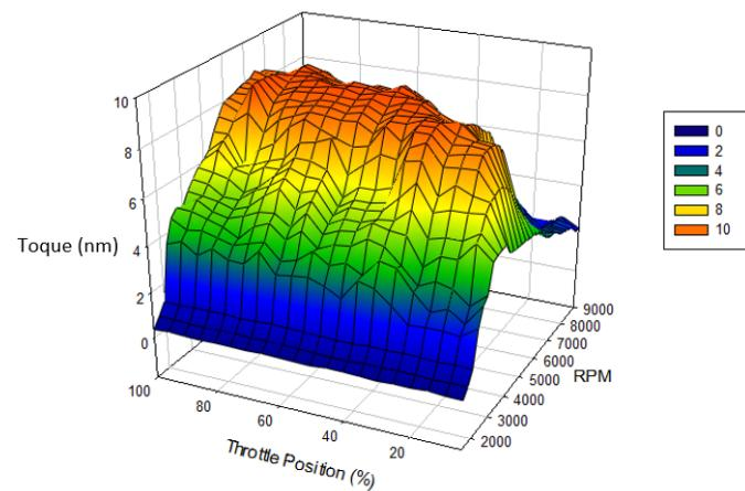
*Figure 15: Generated torque by standard ECU*
