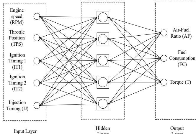
Figure 5: Employed neural network architecture for engine mapping
