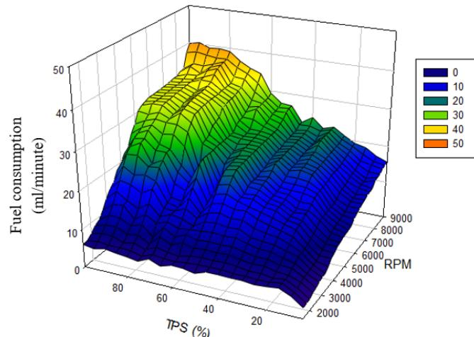
Figure 18: Fuel consumption rate on the standard map engine
