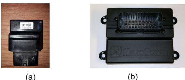
Figure 1: Utilized ECU (a) Standard ECU (b) Modification of engine mapping
