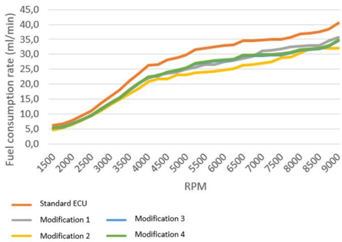
Figure 17: Actual fuel consumption rate test
