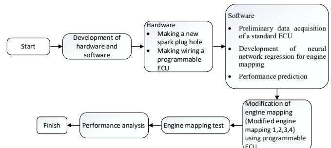
Figure 3: Proposed research flowchart for engine mapping
