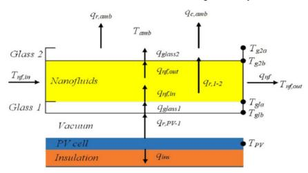
Figure 7: Schematic diagram of using optical filtration nanofluid for the PV/T system
