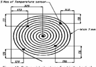
Figure 10: Cotton wick structures fixed in the back of the PV
