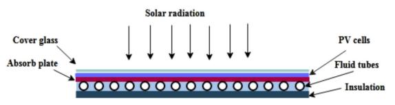
Figure 1: Schematic diagram of the hybrid PV/T system
