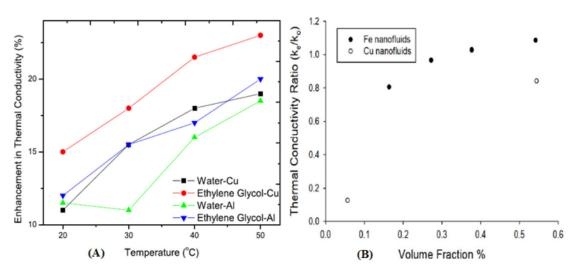
Figure 5: (A) The relationship between Cu and Al with different base fluids and enhancement in thermal energy, (B) The relationship between volume fraction and the thermal conductivity of Fe and Cu nanofluids [74]
