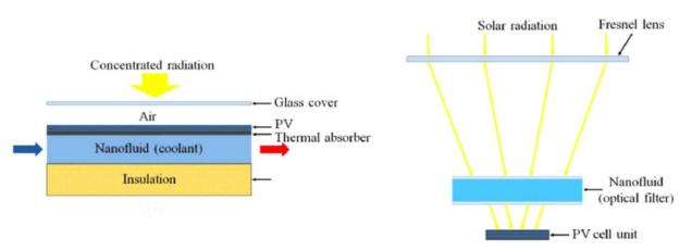
Figure 3: Schematic of the PV/T system with nanofluid as a coolant and spectral [60]
