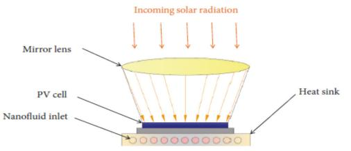
Figure 4: Schematic diagram of the CPV/T system work on nanofluid [64]
