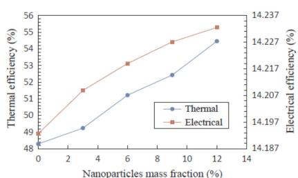
Figure 9: The effect of nanoparticles mass fraction on the efficiency of the PV/T system
