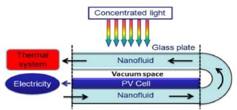
Figure 6: Decoupled PV/T system use nanofluid as a working fluid
