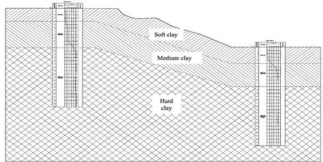
Figure 6: Soil layers based on soil investigation
