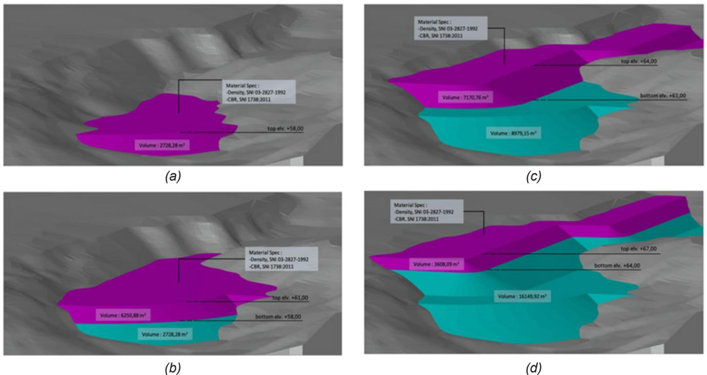
Figure 11: 3D visualization for each elevation of embankment (a) Embankment until elv. +58,00 (b) Embankment until elv. +61,00 (c) Embankment until elv. +64,00 (d) Embankment until elv. +67,00
