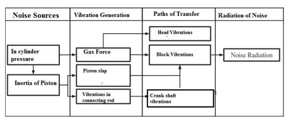
Figure 1: Mechanism of noise generation
