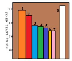
Figure 2: The total noise contribution (8) can be decomposed into contributions due to combustion noise (1), contribution due to piston slap noise (2), contribution due to fan noise (3), contribution to gear operation noise(4), contribution due to pump operations (5), valve noise (6) and other sources (7)
