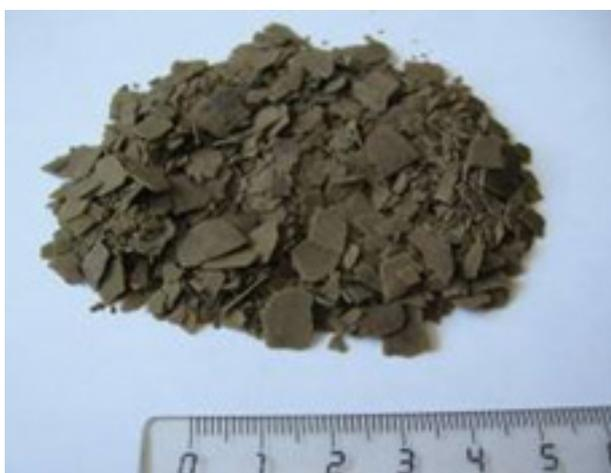
Figure 2: Appearance of scale from well No. 12436
