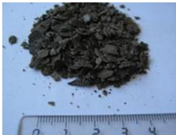
Figure 1: Appearance of scale from well No. 14096
