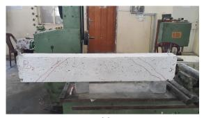
(c) 5cm Figure 16: Modes of failure of specimens without CFRP strips
