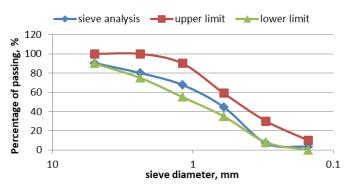
Figure 1: Grading of fine aggregate
