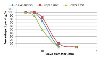
Figure 2: Grading of coarse aggregate
