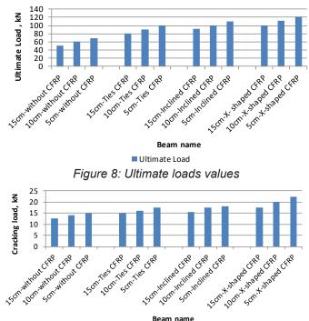
Beam name Cracking load
