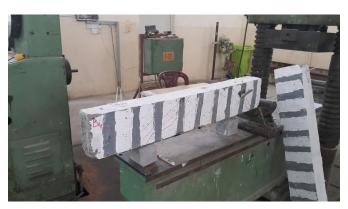
(c) 5cm Figure 17: Modes of failure of specimens with ties CFRP strips
