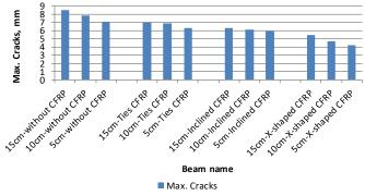
Figure 15: Maximum cracks for the beam specimens
