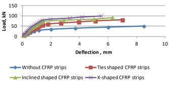
Figure 14: Load-deflection curves for 15 cm spacing between ties reinforcement
