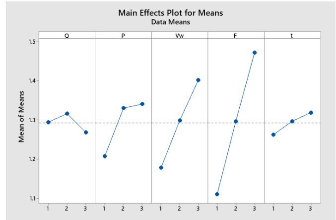
Figure 10: Main effects plot for means of R_q
