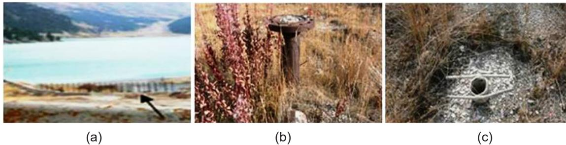
Figure 3: Surface and subsurface objects: a) reinforcing rods protruding from the ground; b) a pipe with a round end; c) H-shaped pipe
