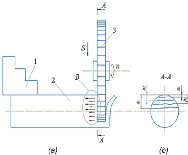
Figure 2: Process flow diagram of thermo-frictional cutting with pulsed cooling (a – front view; b – incision A-A; S – feed; n – disk rotational speed; h1, h2, h3, h4 – distance of temperature distribution deep into the workpiece from the contact; B – temperature distribution from the end surface; 1 – three-jaw chuck; 2 – work piece; 3 – circular saw)
