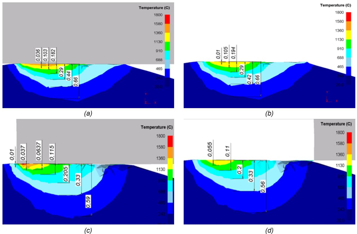
Figure 5: Models of temperature change in one revolution of the disk in the heating and cooling zones, with  $L_1=18$  mm;  $L_2=14$  mm (a,b -  $n_{\partial}=2000$  r/min; c,d -  $n_{\partial}=3000$  r/min;  $S = 120$  mm/min;  $\delta = 2$  mm; a,c – heating zone models  $L_1=18$  mm; b,d – cooling zone models  $L_2 =14$  mm)
