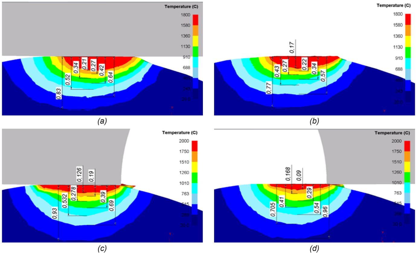
Figure 6: Models of temperature change in one revolution of the disk in the heating and cooling zones, with  $L_1=26$  mm;  $L_2=6$  mm (a,b -  $n_\delta=2000$  r/min; c,d -  $n_\delta=3000$  r/min;  $S=120$  mm/min;  $\epsilon=2$  mm; a,c – models of heating zone  $L_1=26$  mm; b,d – models of cooling zone  $L_2=6$  mm)
