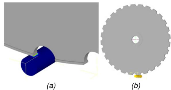
Figure 3: Fragment of a cut with a circular saw and a view of a model of a disk and a workpiece with a distributed mesh of finite elements (a - a fragment of a cut off with a circular saw; b - a view of a disk with workpiece)
