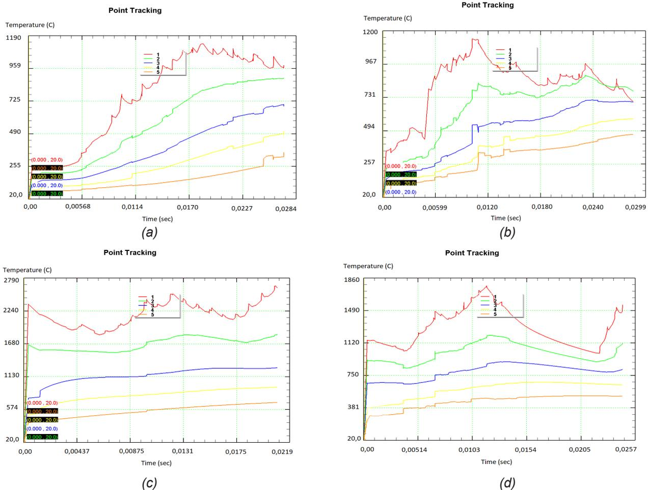
Figure 4: Graphs of the temperature distribution depending on the time of the segment with the marking of the contact layer deep into the workpiece for different sizes  $L_1$  и  $L_2$  (a,c -  $n_0 = 2000 \text{ r/min}$ ; b,d -  $n_0 = 3000 \text{ r/min}$ ; a, b -  $L_1 = 18 \text{ mm}$ ,  $L_2 = 14 \text{ mm}$ ; c,d -  $L_1 = 26 \text{ mm}$ ,  $L_2 = 6 \text{ mm}$ ;  $S = 120 \text{ mm/min}$ )
