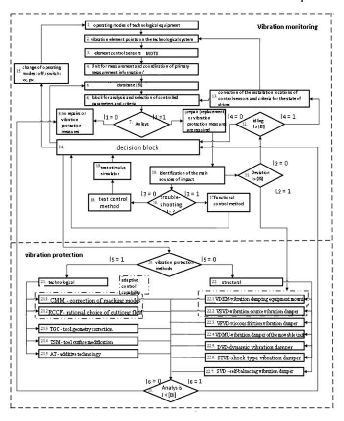
Figure 3: Block diagram of the algorithm for the selection and rational use of structural and technological methods of vibration protection of vehicle elements in order to increase the efficiency of machining based on the results of functional and test vibration monitoring (lj-bits of information)
