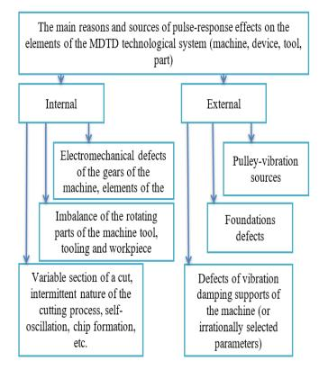
Figure 1: The main causes and sources of impulse - vibration effects on MDTD elements
