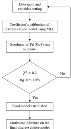
Figure 3: Model calibration flowchart
