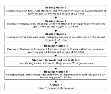
Figure 3: Flow process map of Brazing process
