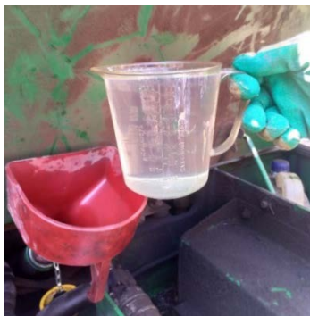
Fig. 27. A graduated measuring cup for refueling the fuel tank of forwarders
