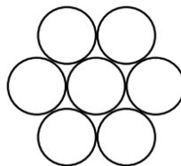
Figure 1: Cross section of a seven-wire reinforcing rope structure
