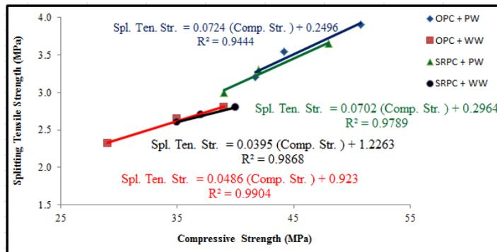
Fig. 9 Correlation between (compressive and tensile strength)
