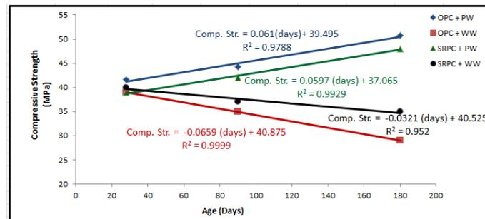
Fig. 5 Change of compressive Strength with time.
