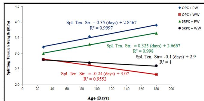
Fig. 6 Change of splitting Tensile Strength with time.
