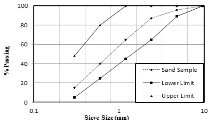
Fig. 1 Fine aggregate grading.
