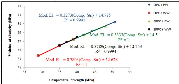
Fig. 12 Correlation between (compressive strength and modulus of elasticity).
