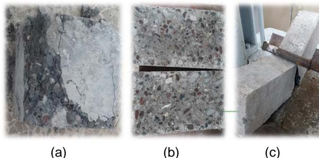
Fig. 14 Failure in Specimens for (a) compression (b) splitting (c) flexural
