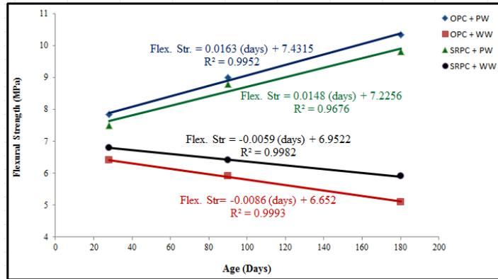
Fig.7 Change of Flexural Strength with time
