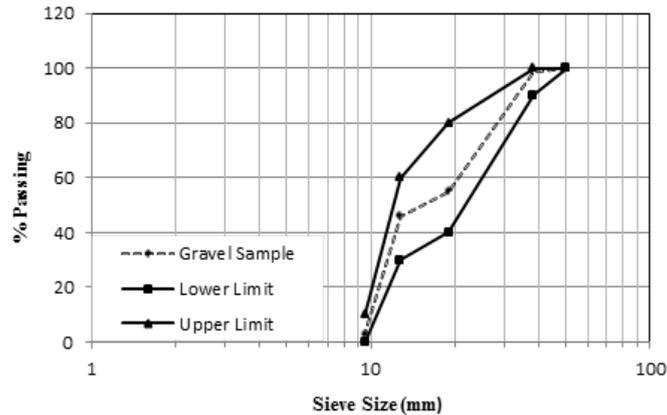
Fig. 3 Grading of coarse aggregate
