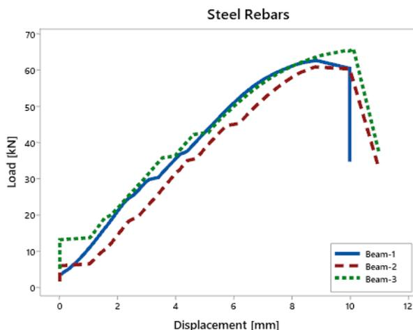
Fig. 5. Load-Displacement graph of the concrete beams reinforced with steel rebars.
