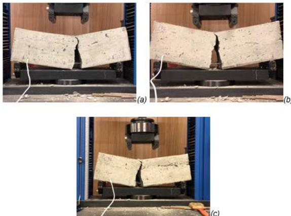
Fig. 9. Failure of the Nickel-Titanium reinforced beams in the flexural strength test. (a) beam-4; (b) beam-5; (c) beam-6.
