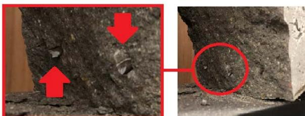
Fig. 7. Detail of the steel rebar fractures after completion of the test.
