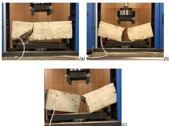
Fig. 6. Failure of the concrete beams reinforced with steel rebars in the flexural strength test. (a) beam-1; (b) beam-2; (c) beam-3.
