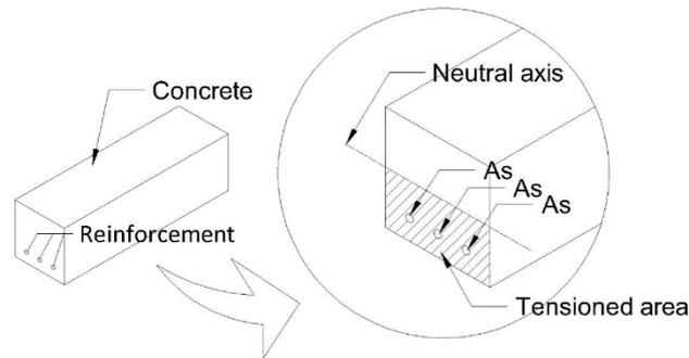
Fig. 3. Definition of the tensile area in the cross section
