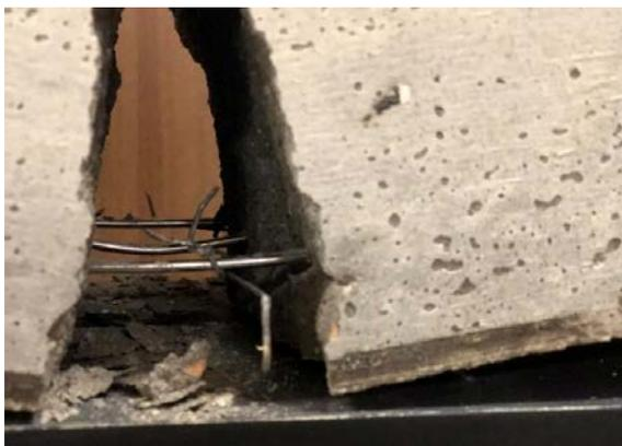
Fig. 10. Detail of the Nickel-Titanium rebars after completion of the test.
