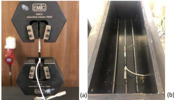
Fig. 4. Device with extensometer for checking the development of internal forces during the test. (a) calibration of the device on a universal testing machine; (b) inserting the device into the reinforcing rebars.
