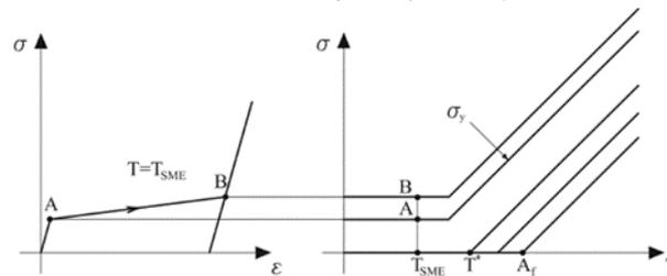
Fig. 1. Stress-Strain Shape Memory theoretical graph [10]
