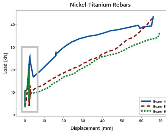
Fig. 8. Load-Displacement Graph of the concrete beams reinforced with Nickel-Titanium rebars
