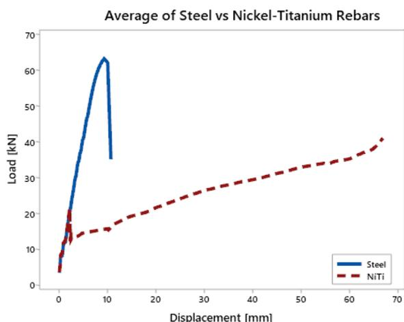
Fig. 11. Comparison of Load-Displacement curves of the averages of the reinforcements used.
