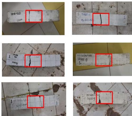
Fig. 7. Crack pattern of flexural strength test of specimens
