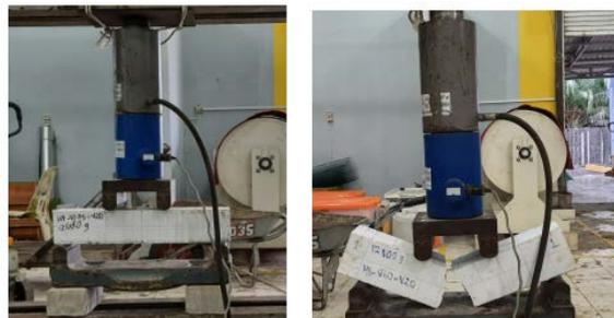
Fig. 6. Test flexural strength set-up
