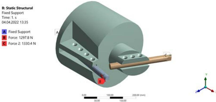
A - rigid sealing of the end of the body of the boring bar; B - cutting force components when boring a hole with a diameter of 325 mm; C - components of the cutting force when boring a hole with a diameter of 295mm.
