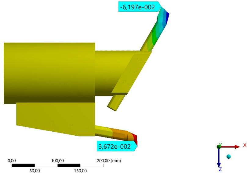
Fig. 17. Radial deformations at the tips of cutter blades
