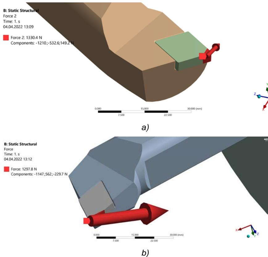
a) - 60° for boring a hole with a diameter of 295 mm; b) - 80° for boring a hole with a diameter of 325mm
