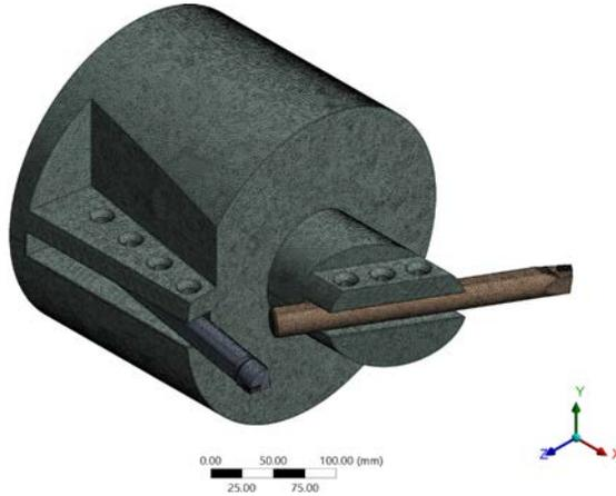
Fig. 6. Boring bar finite element mesh
