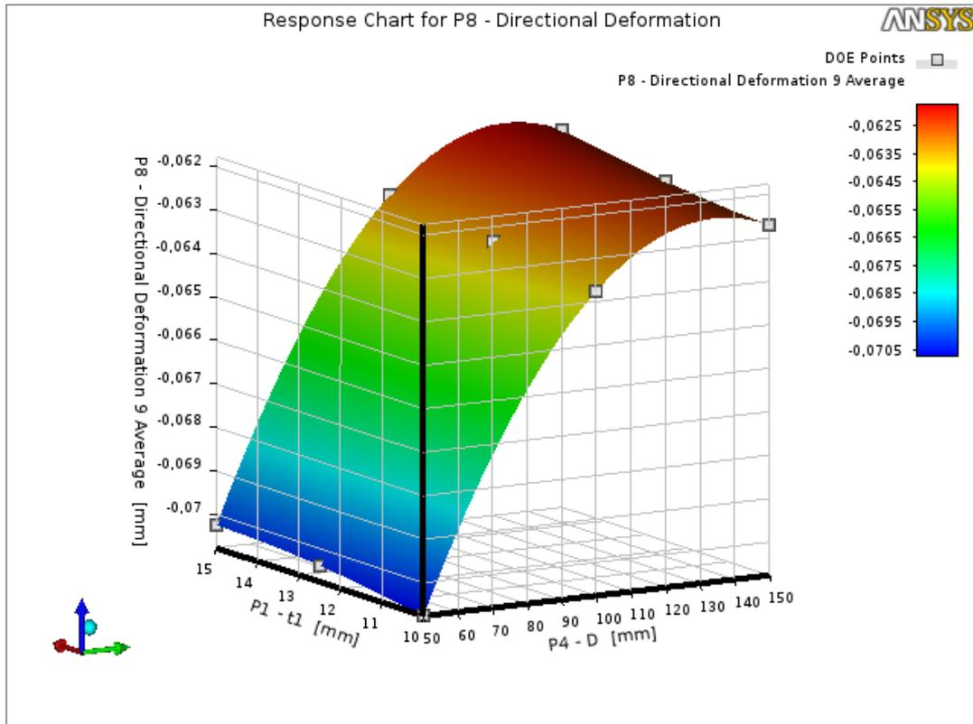
Fig. 13. Response surface of radial displacement from two parameters
