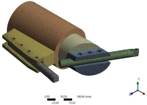
Fig. 15. Rational finite element grid of the boring bar
