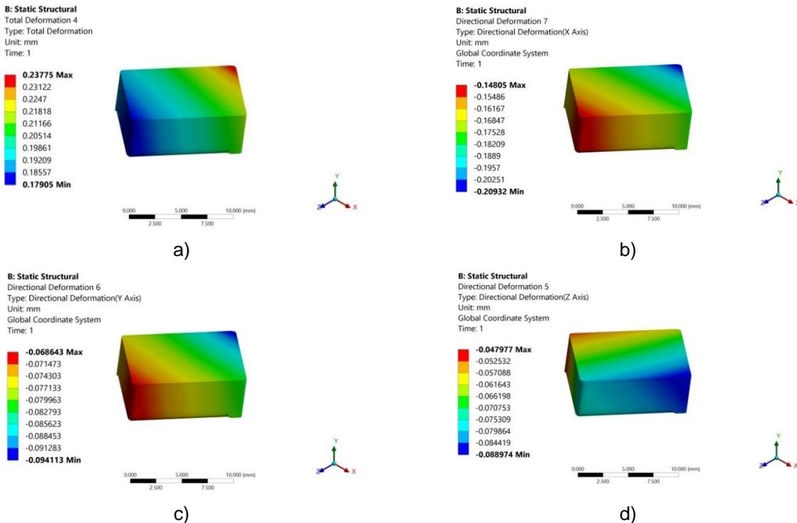
a - resulting deformation; b - X - in the axial direction; c - Y - in the circumferential direction; g - Z - in the axial direction
