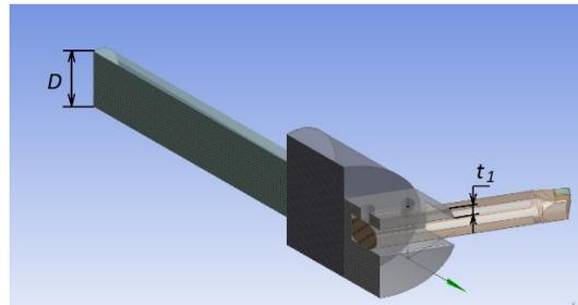
Fig. 11. Parametric model of the boring bar
