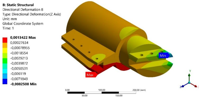
Fig. 16. Deformation of the boring bar body
