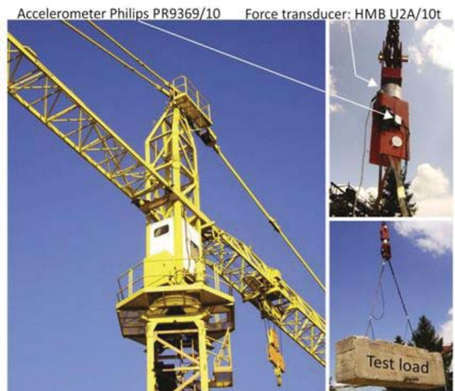
Figure 5: Testing the POTAIN-744E tower crane
