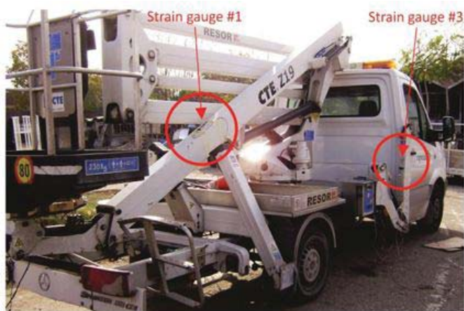
Figure 7: Testing the elevating work platform
