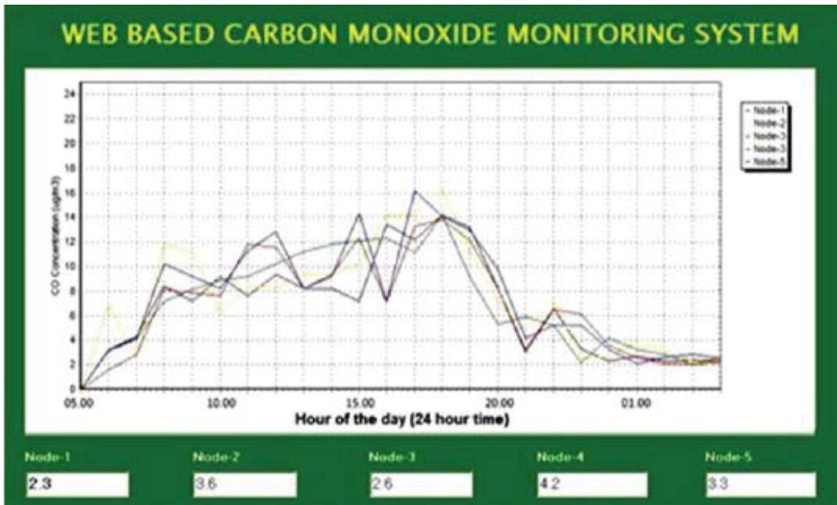
Figure 3: CO measurement at sensor node as displayed in real-time
