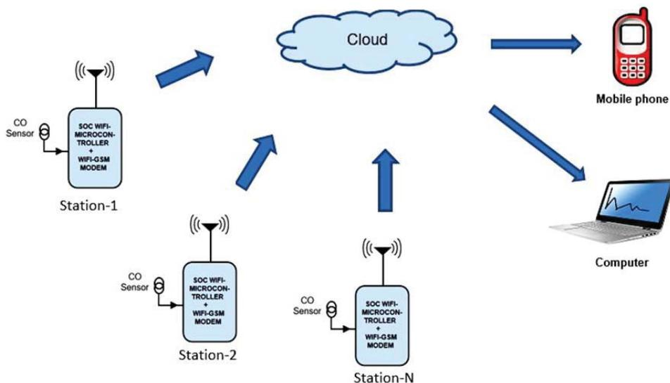
Figure 1: Carbon monoxide network for the online system
