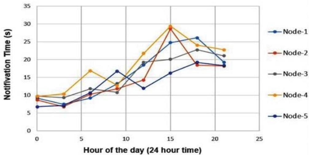
Figure 5: Results of testing for warning time from sensor nodes to the cellular phone
