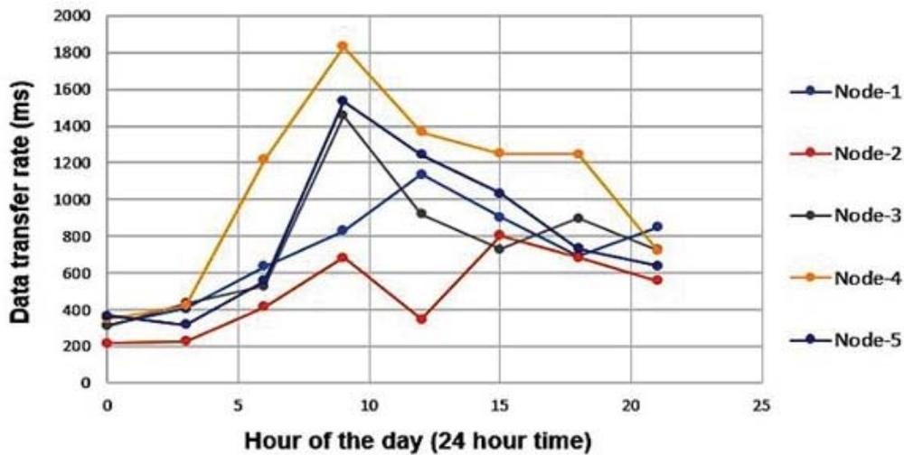
Figure 4: Results of testing for data transfer rate from sensor nodes to the web server
