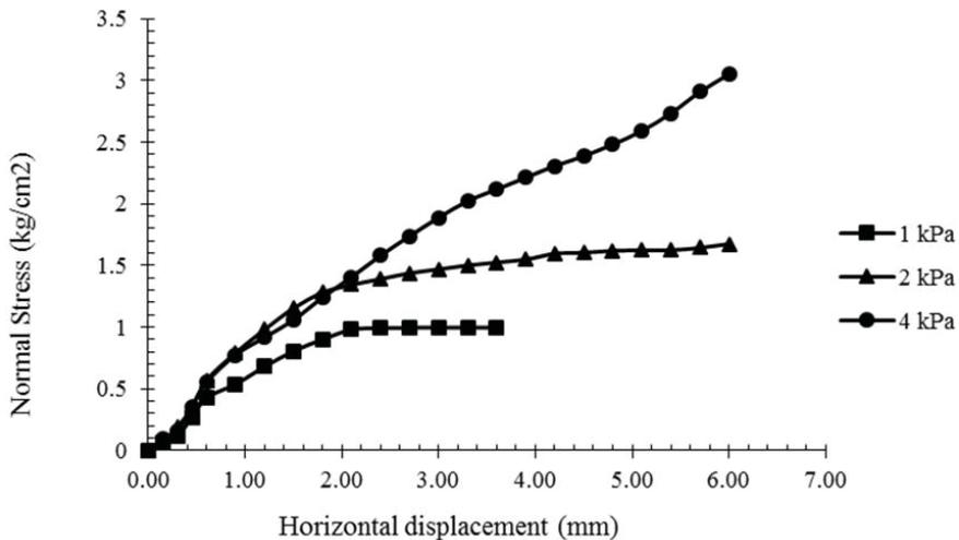
Figure 5: Stress and strain soil mixture 1 with 7 day curing periode from direct shear test
