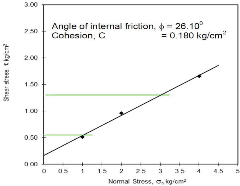
Figure 3: The soil– pile friction resistance
