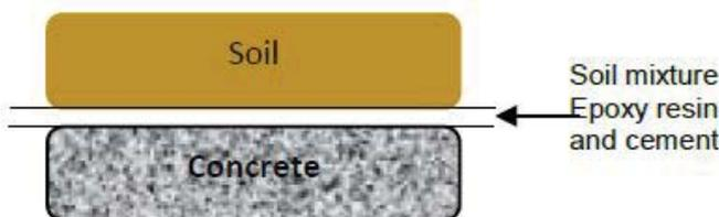
Figure 2: Schematic of laboratory sample to simulate soil and pile interface friction
