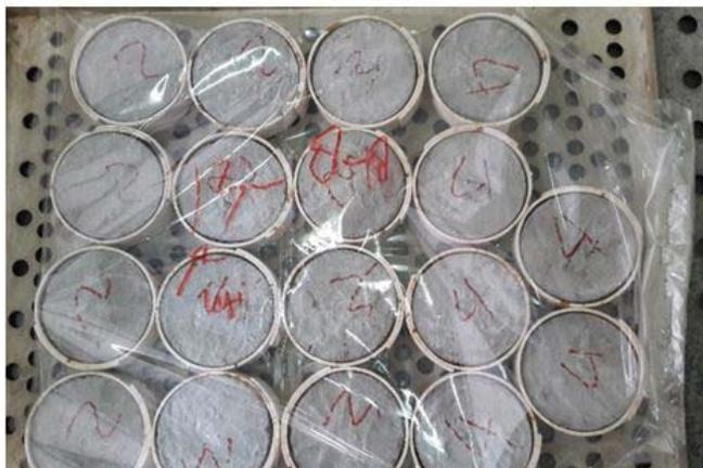
Figure 1: Preparation of Concrete Sample
