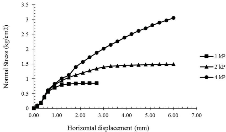
Figure 4: Stress and strain soil mixture 1 with 3 day curing periode from direct shear test
