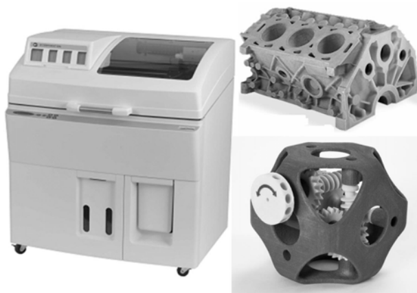
Figure 10. 3D printer with printed machine part and assembly
