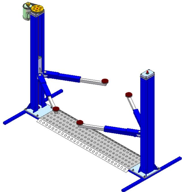
Figure 8. Main assembly of electromechanical two post lifts
