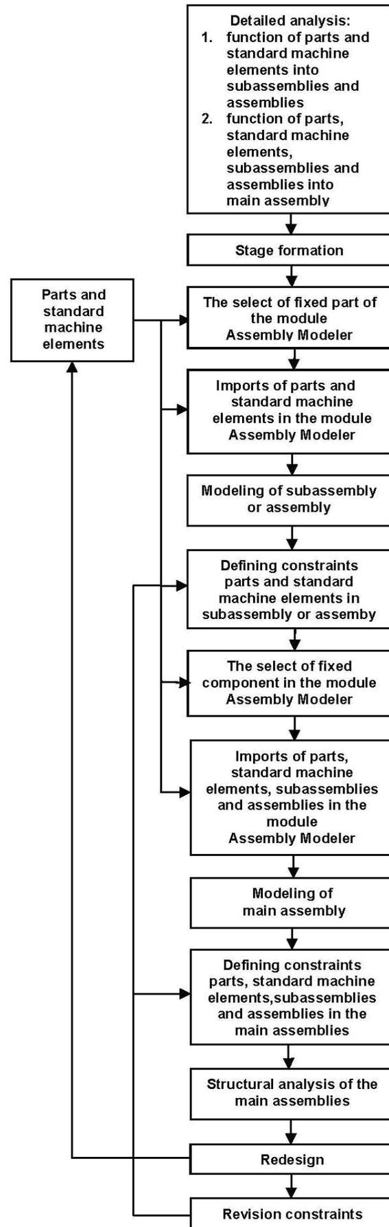
Figure 4. Structural diagram modeling higher levels
