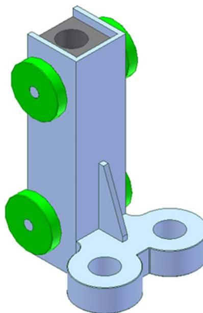
Figure 6. Mobile carrier console - subassembly
