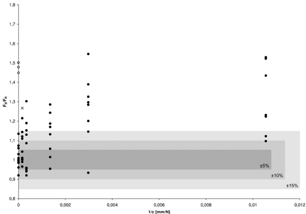
Figure 9. Ratios of actual and theoretical values of force depending on stiffness of structure
