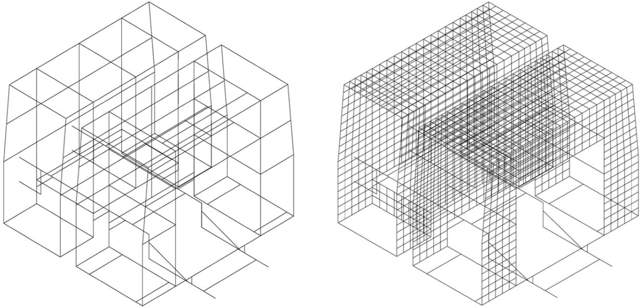
Figure 1. FEM model of one superstructure variant (beam and plate finite elements)
