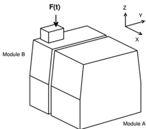
Figure 6e) exciter attached to fixed superstructure in Z direction
