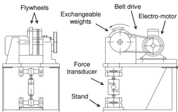
Figure 3. Mechanical vibration exciter
