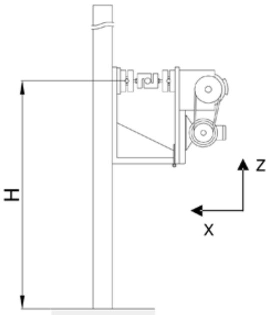
Figure 6c) exciter attached to post
