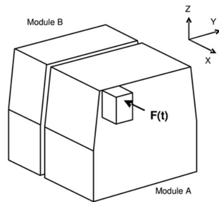
Figure 6d) exciter attached to fixed superstructure in X direction
