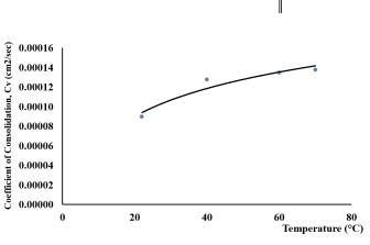
Figure 5: The relationship between the consolidation coefficient (Cv) and temperature variations
