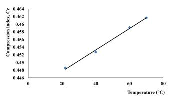
Figure 3: Relationship of compression index (Cc) and temperature variation
