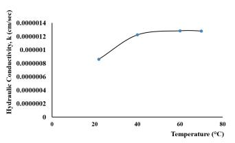
Figure 8: Relationship between soil permeability coefficient (k) and temperature variations
