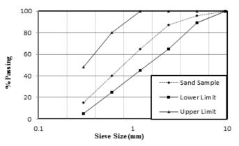
Fig. 1 Fine aggregate grading.
