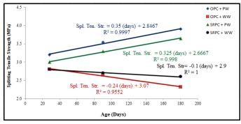
Fig. 6 Change of splitting Tensile Strength with time.
