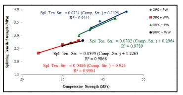
Fig. 9 Correlation between (compressive and tensile strength)
