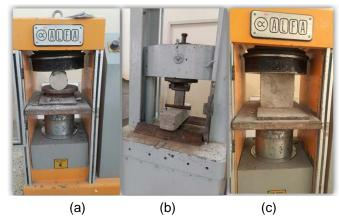
Fig. 4 Experimental setup for (a) compression test (b) Splitting tensile Test (c) flexural test
