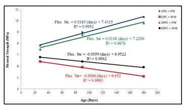
Fig.7 Change of Flexural Strength with time
