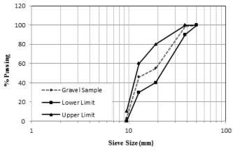
Fig. 3 Grading of coarse aggregate
