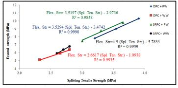
Fig. 10 Correlation between (flexural and tensile strength)
