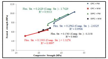
Fig. 8 Correlation between (compressive and flexural strength)
