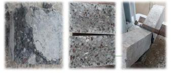
(a) (b) (c) Fig. 14 Failure in Specimens for (a) compression (b) splitting (c) flexural 1342
