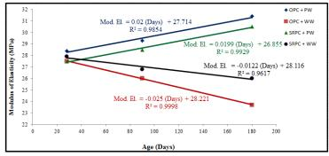
Fig. 11 Change of modulus of elasticity with time.
