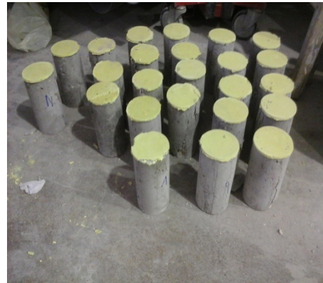
b) Capping concrete cylinders
