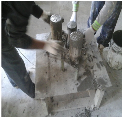
a) Casting and compacting cylinders
