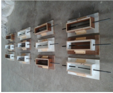
a) Steel bar inside the wooden mold
