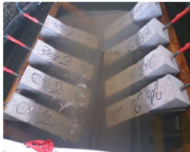
b) Connecting the anode and cathode wires with the device
