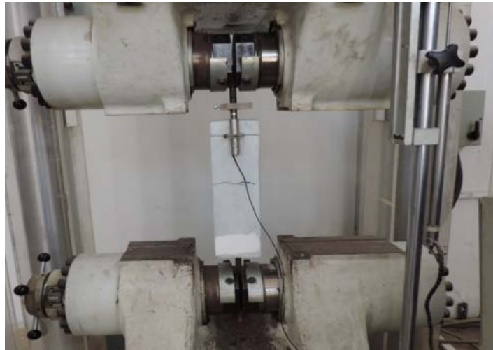
Figure 6. The pull-out test setup
