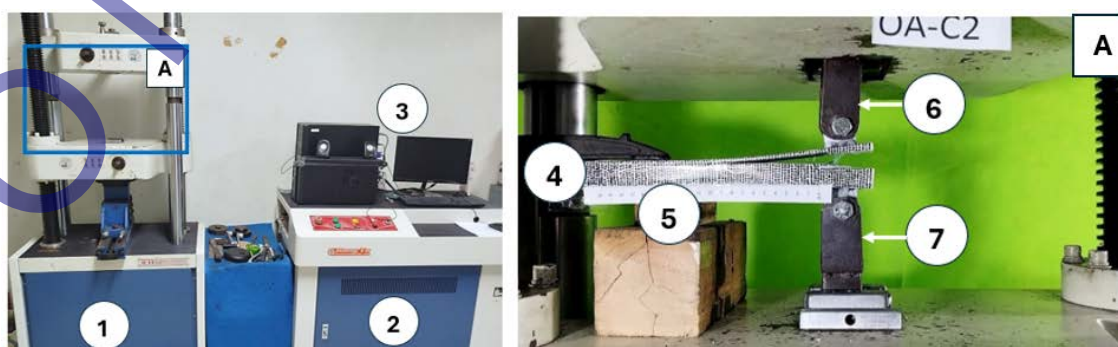
Fig. 4. Experimental setup for mode-I loading test: 1) testing machine; 2) power pack; 3) PC/computer; 4) clamp; 5) sandwich beam specimen; 6) upper hinge; 7) lower hinge
