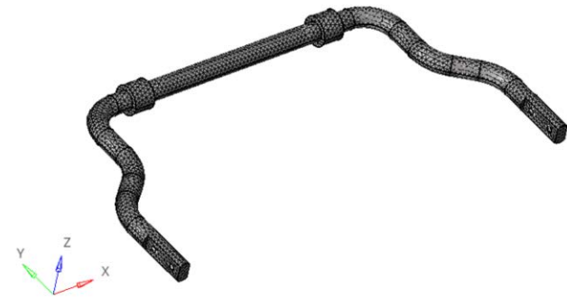
Fig 8. Mesh topology of the anti-roll bar
