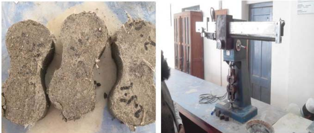
Figure 10: Briquette Samples (left) & Briquette Testing Machine (Right)
