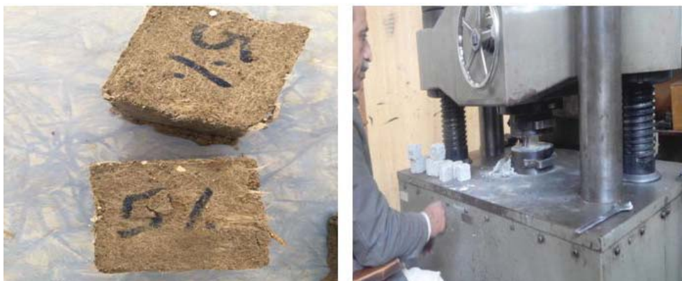
Figure 8: Cube Samples (Left) & Universal Testing Machine (Right)
