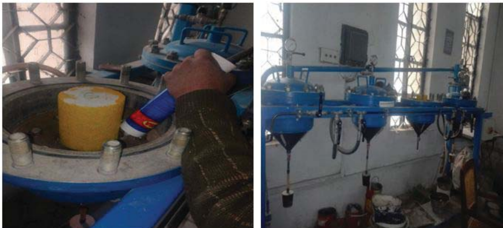
Figure 14: Cylinder Samples (Left) & Permeability Apparatus (Right)
