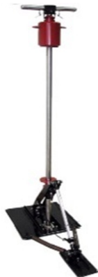
Figure 2: General view of the coupling coefficient of friction meter portable CGCp-2M
