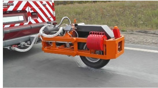
Figure 3: Car installation type EGMD-2 (Evenness and Grip Monitoring Device)
