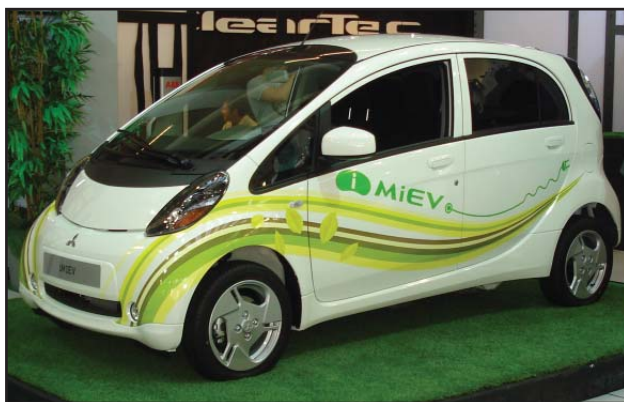
Figure 5. Typically EV, as the producer MiEV Mitsubishi Motors [08], is shown at the Belgrade automotive Fair in 2011., has exterior dimensions less than 3.5 x 1.5 m and 35 kW AC electric motor, developing a maximum speed of 130 km/h and Li-ion accumulators that allow a maximum range to 150km
