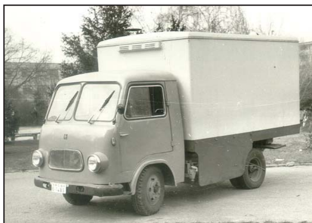
Figure 3. The first EV in the country had DC series motor 27 kW and could reach speed of 42 km/h, battery voltage 108 V, a capacity of 350 Ah which allowed radius of the 48 km
