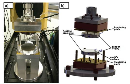
Figure 2: An instruments a) Instron 5567 used for measurement, b) image of test stand in SolidWorks.
