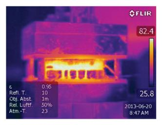
Figure 4: Thermographic image of the heating surfaces
