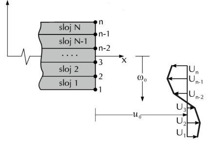
Figure 1: Displacement through the thickness of the plate
