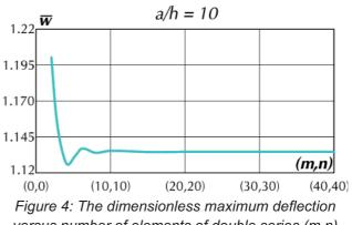
Figure 4: The dimensionless maximum deflection versus number of elements of double series (m,n) for side-to-thickness ratio a/h=10 and cross-ply 0°/90°/0° laminate
