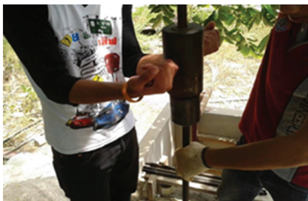
Figure 6: Kunzelstab penetration test
