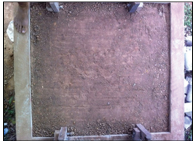
Figure 4: Soil preparations in testing tank
