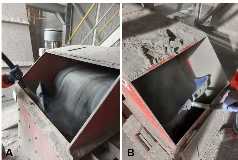
Fig. 5. Sampling with a special shovel: A) from input conveyor belt; B) from output conveyor belt
