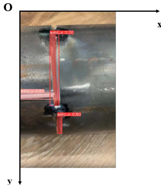
Fig. 5. The coordinates of the welds are continuously updated
