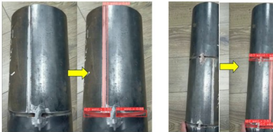
Fig. 4. Results of identifying horizontal and vertical welds in real-time
