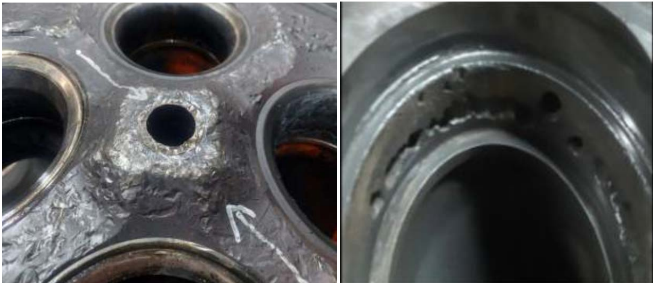
Fig. 2. of the cylinder head crack
