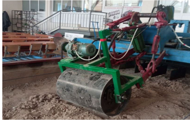
Fig. 3. Fragment of an experiment to establish roadbed compaction patterns on a physical simulation setup
