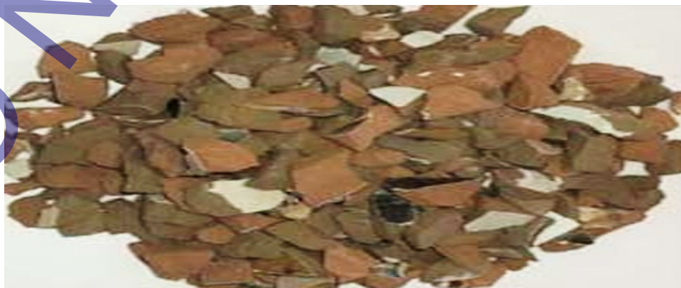
Fig. 1. Ceramic recycled coarse aggregates (RCA)
