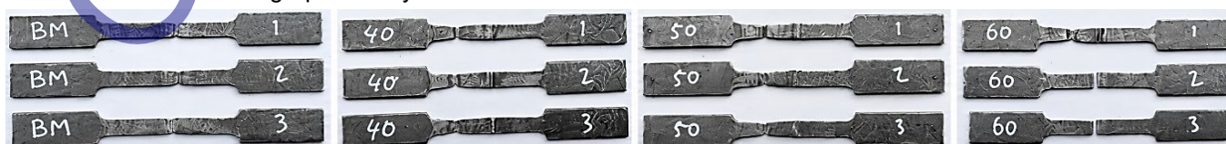
Fig. 5. Tensile specimens after testing: Base Metal (BM) and GMAW-welded specimens at welding speeds of 40, 50, and 60 cm/min
