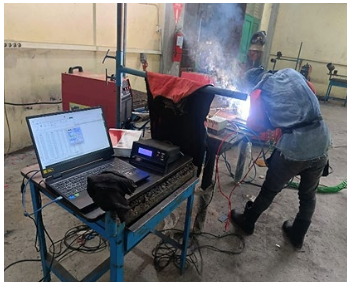
Fig. 3. Shielded metal arc welding (SMAW) process
