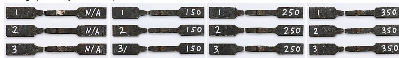
Fig. 8. Post-fracture tensile specimens under different preheating conditions
