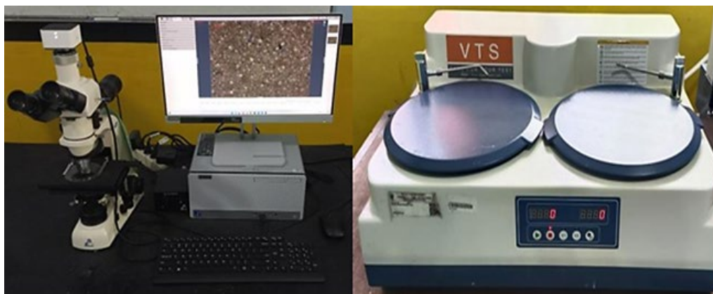
Fig. 6. Metallographic testing machine and metallographic polishing machine
