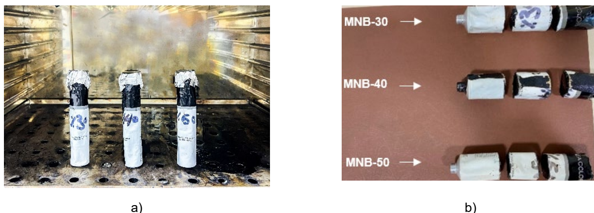
Fig. 4. Storage stability test: NB-modified binders in the aluminum tubes during thermal conditioning phase (a) and sectioning phase (b)
