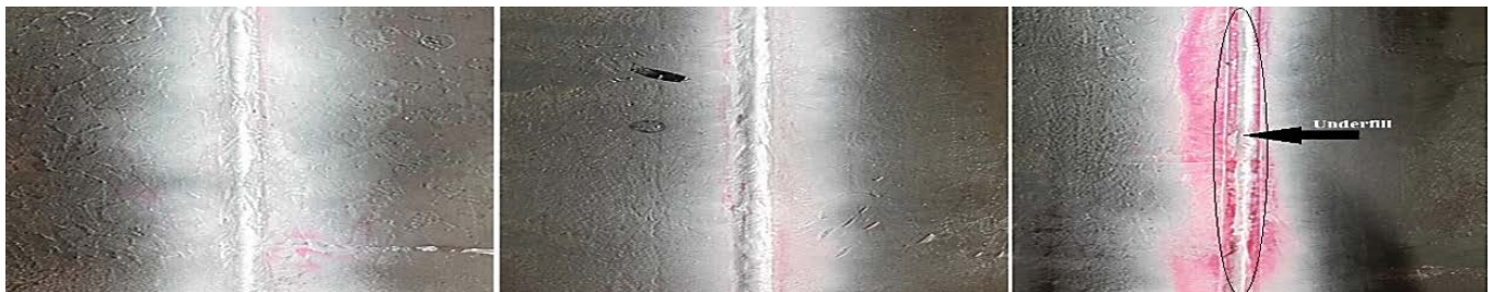
Fig. 4. Visual inspection and liquid penetrant testing results of joints welded at (a) 40, (b) 50, and (c) 60 cm/min. The arrow and ellipse indicate localized underfill in the 60 cm/min joint
