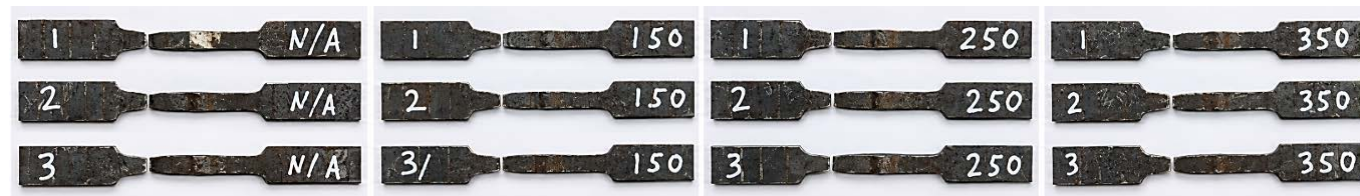
Fig. 8. Post-fracture tensile specimens under different preheating conditions
