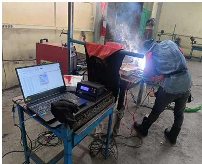
Fig. 3. Shielded metal arc welding (SMAW) process
