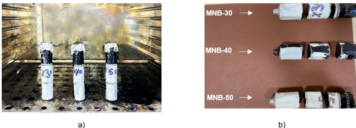
Fig. 4. Storage stability test: NB-modified binders in the aluminum tubes during thermal conditioning phase (a) and sectioning phase (b)
