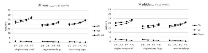
Figure 8: Calculated results for the heating  $(Q_p)$ , cooling  $(Q_o)$  and total annual energy need  $(Q_{total})$  for Athens and Madrid; Uwall = 0.10 W/m<sup>2</sup>K, Uroof = 0.10 W/m<sup>2</sup>K, Ufloor = 0.135 W/m<sup>2</sup>K
