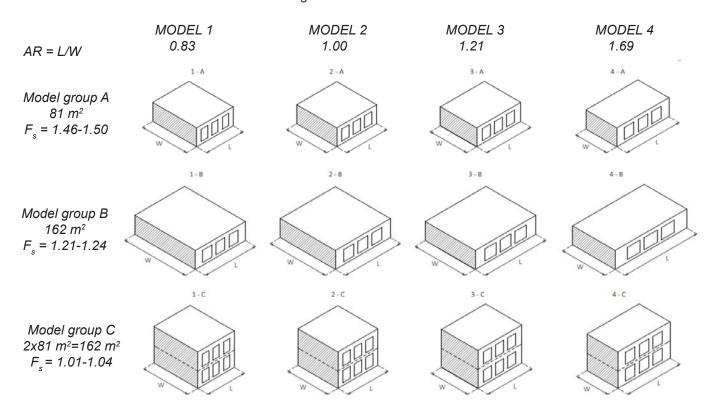
Figure 4: Schematic presentation of the analysed house models
