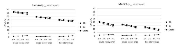
Figure 7: Calculated results for the heating (Qh), cooling (Qc) and total annual energy need (Qtotal) for Helsinki and Munich; Uwall = 0.10 W/m<sup>2</sup>K, Uroof = 0.10 W/m<sup>2</sup>K, Ufloor = 0.135 W/m<sup>2</sup>K
