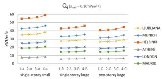
Figure 5: Calculated transmissions losses for all models;  $U = 0.10 \text{ W/m}^2\text{K}$
