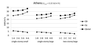
Figure 9: Calculated results for the heating  $(Q_h)$ , cooling  $(Q_o)$  and total annual energy need  $(Q_{total})$  for Athens;  $Uwall = 0.20 \ W/m^2 K$ ,  $Uroof = 0.20 \ W/m^2 K$ ,  $Ufloor = 0.25 \ W/m^2 K$
