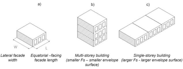
Figure 2: Schematic presentation of the building aspect ratio (a) and a differing shape factor for two different types of rectangular buildings (b-c)
